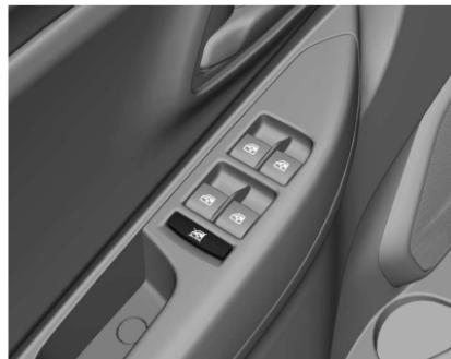
Pulse el interruptor
