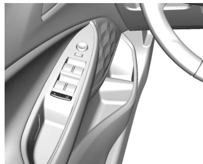
Pulse el interruptor
