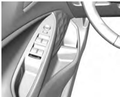
Pulse el interruptor
