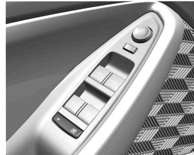
Pulse el interruptor
