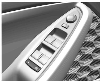
Pulse el interruptor
